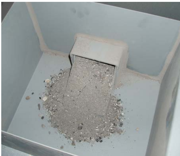
Figures 23 and 24: Ash container and discharge of ashes through a feed screw.
