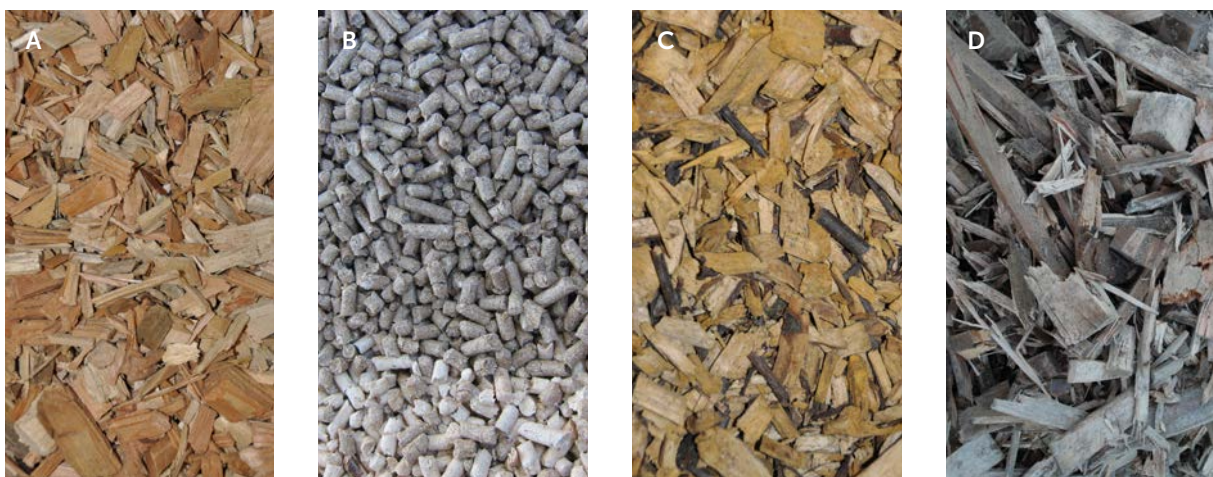
Figure 9: Various types of biomass fuel: (A) forestry chips without bark, (B) wood pellets, (C) forestry chips with bark (full chipped trees) and (D) untreated, non-polluted wood waste
